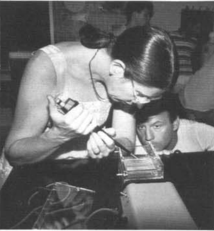
Teachers prepare to separate DNA fragments using gel electrophoresis.
